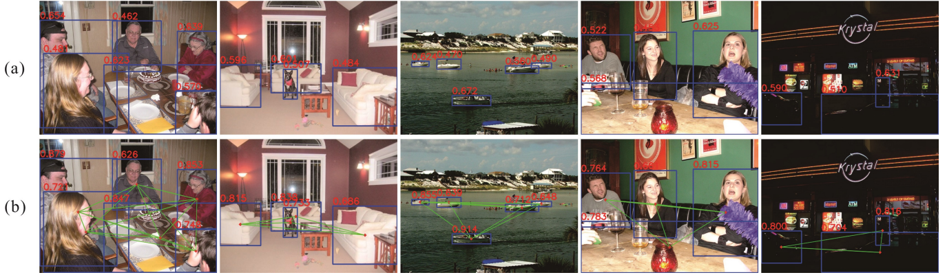
Figure 3. Some examples of learned class-based graph representation from our ClassGCN. The red numbers are the predicted classification scores; the blue boxes are the predicted bounding boxes; and the green graph structures are the graph relations with various weights. Row (a) is the detection visualization of the base model [24], and Row (b) by means of our ClassGCN. Our method outperforms baseline with better classification scores due to the help of graph relations.
